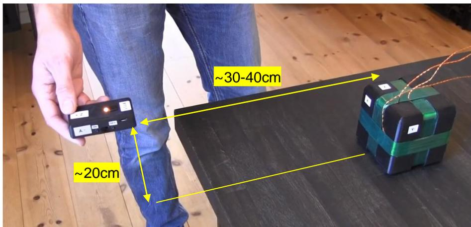
When the correct calibration position is found, the sensor LED will stop flashing yellow and light up constantly yellow. Then push the sensor button, and if start up calibration is successful, the LED turns green, and the sensor should now be visible in the AmfiTrack Viewer software.
