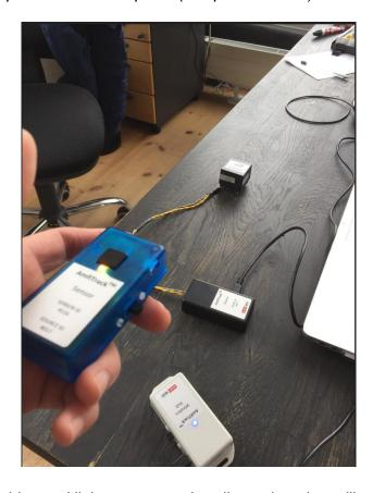
The sensor will stop flashing and light up constantly yellow, when the calibration position is correct. Then push the button of the sensor, and the sensor should be visible in the AmfiTrack Viewer software.
